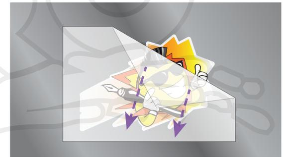
Remove the masking paper by pulling down against itself, leaving just the applied vinyl.
